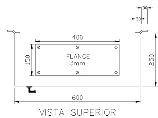
OBS: FIXAR O QUADRO NA PAREDE COM PARAFUSOS EM AÇO INOX
